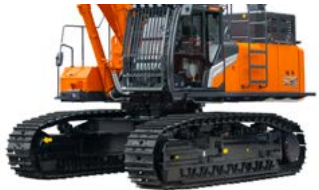
The robust undercarriage of the ZX530LCH-7.
