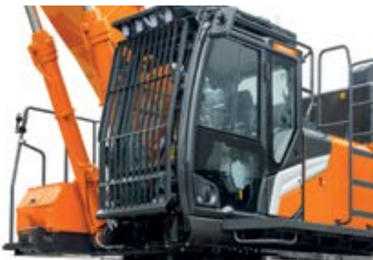
Front guard, top guard and four cab lights are standard on the ZX530LCH-7.
