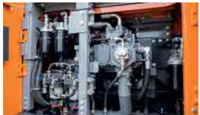
A fuel saving of up to 22% is achieved with the HIOS V hydraulic system.
