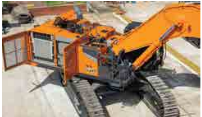
Components are conveniently accessible for daily maintenance.
