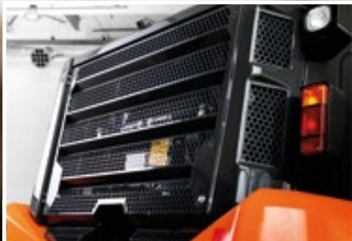
New rear grill protects radiator compartment.
